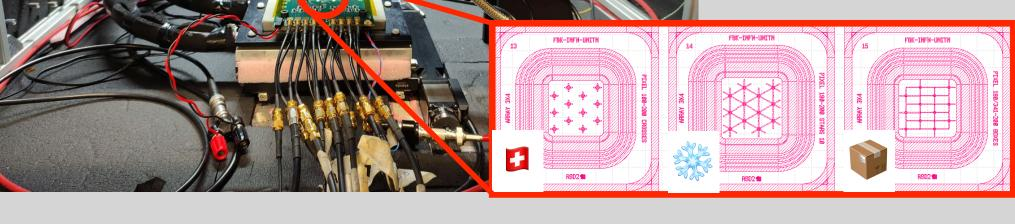
Signal properties are used for **position reconstruction** of laser shots
