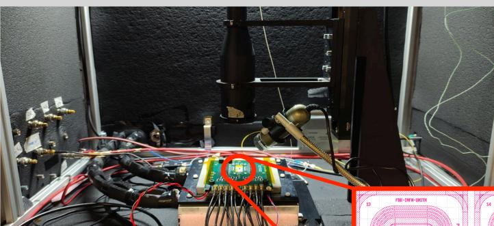
Three sensors have been selected from the **second RSD production**: 700x700 µm active area, 200 µm pitch and 3x4 **AC pads with different layouts** (Swiss crosses, flakes and boxes)
