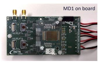
Main demonstrator (MD1) chip of (1.2×1.2)cm<sup>2</sup> with  $512\times512$  fully depleted monolithic pixels with  $25\mu m$  pitch.
