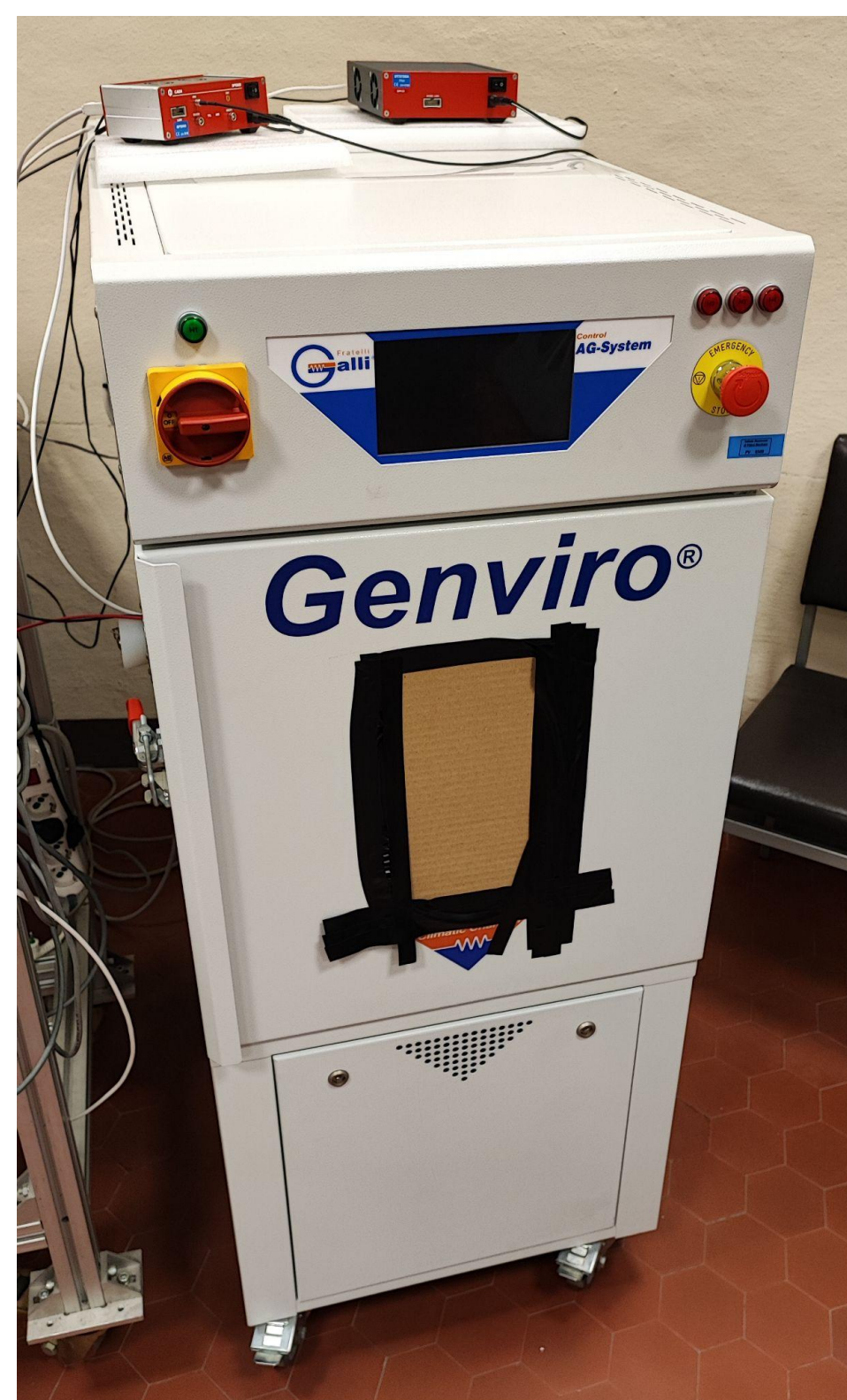
Fig. 1: Climatic Chamber with the SP5600 Power Supply and the DT5720A digitizer on top of it.
