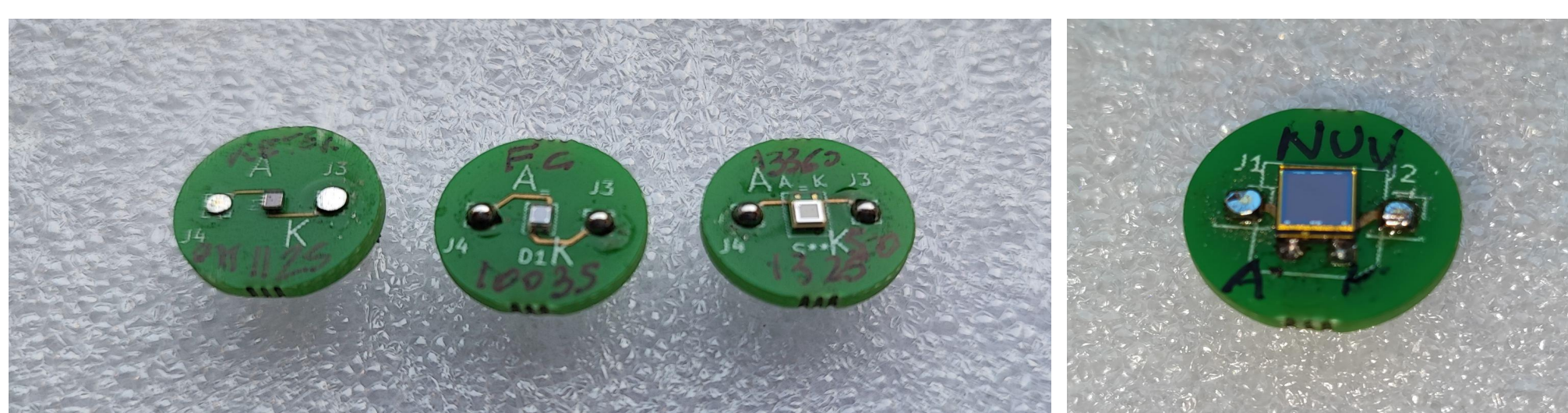
Fig. 3: Picture of the four SiPMs mounted on a custom PCB adapter.
