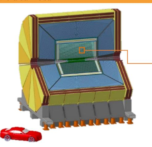
he IDEA general-purpose detector concept has been designed to study electron-positron collisions in a wide energy range provided by a very large circular leptonic collider [1,2].
