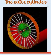
Assembly of the spoke with the inner and intermediate rings.
