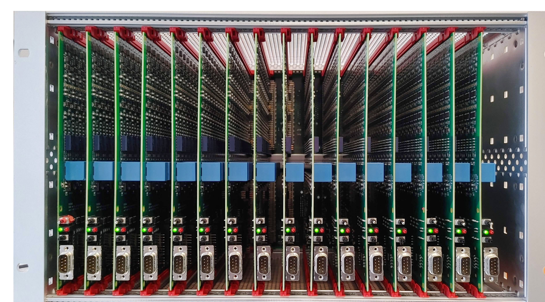
Figure 8: Full crate with 16 boards (192 channels)
