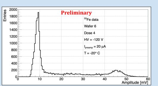
• **First peak** and **second peak** are extracted from the spectrum and used to calculate the gain for the <sup>55</sup>Fe X-rays
