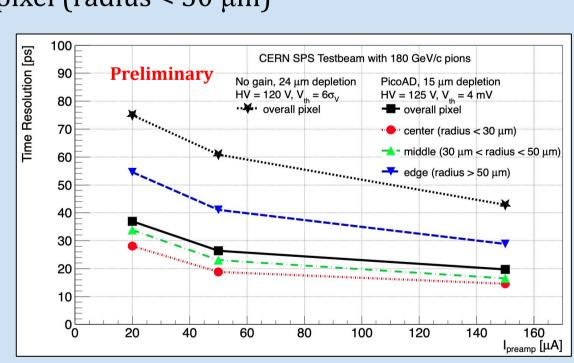
The gain layer improves the efficiency and the time resolution
