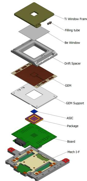
The concept of the GPD as a sealed gas cell with a Gas Electron Multiplier and a finely pixelated custom ASIC readout was conceived 15 years ago (NIM-A-566-2006, 552-562) and its maturity was key in the adoption by NASA for IXPE.
