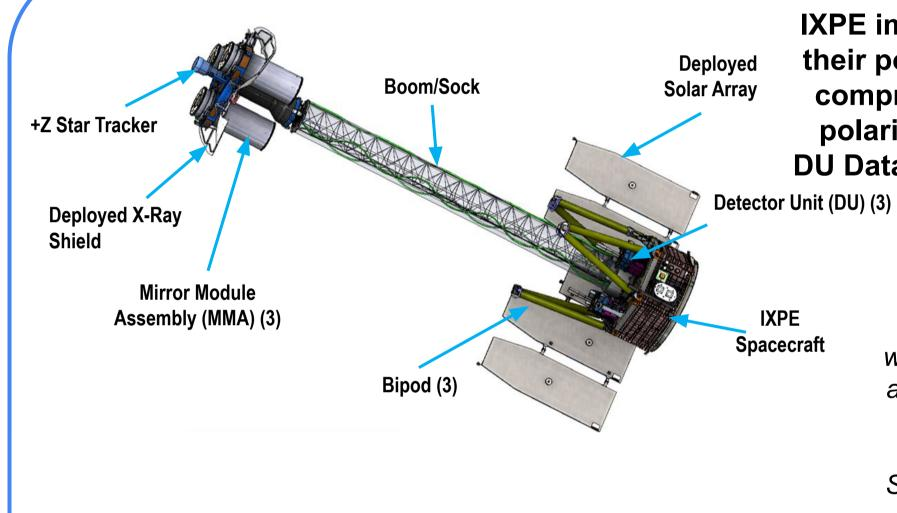
IXPE images X-rays in the 2-8 KeV range and measures their polarization using three identical telescopes each comprised of a Mirror Module Assembly (MMA) and a polarization sensitive Detector Unit (DU) at its focus. DU Data are handled by the Detector Service Unit (DSU).
