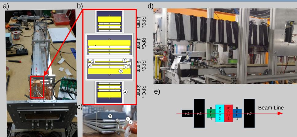
Figure 1. a). Internal arrangement of the four chambers. b) Cross section of the four chambers arrangement. c) RPC chamber: ① aluminum and ② glass electrodes, ③ plastic support bar, ④ aluminum tube. d) Panoramic view of the setup in the beam line, showing the tRPC chambers gas box, surrounded by the heating wire, and the last scintillator of the telescope. e) Cross section of the scintillator and tRPC counters in the beam line.
