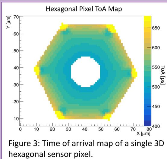
Figure 3: Time of arrival map of a single 3D hexagonal sensor pixel.
