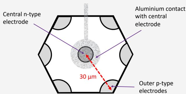
Figure 2: Simple illustration of a single pixel of a 3D hexagonal sensor.
