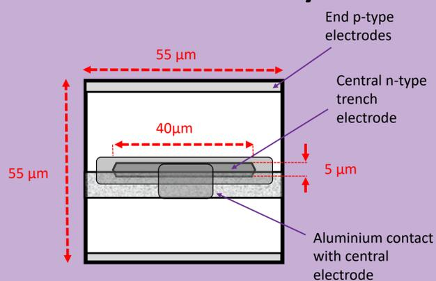
Figure 5: Simple illustration of a single pixel of a 3D trench sensor.
