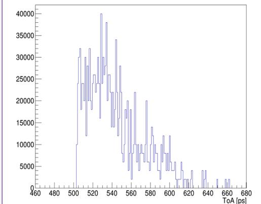
Figure 4: Time of arrival histogram of a single 3D hexagonal sensor pixel
