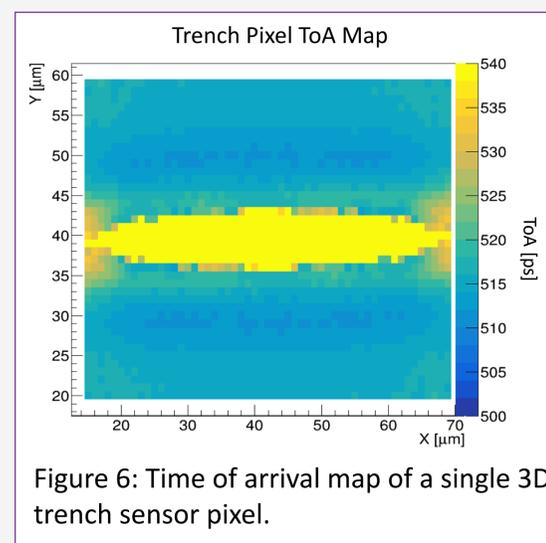
Figure 6: Time of arrival map of a single 3D trench sensor pixel.
