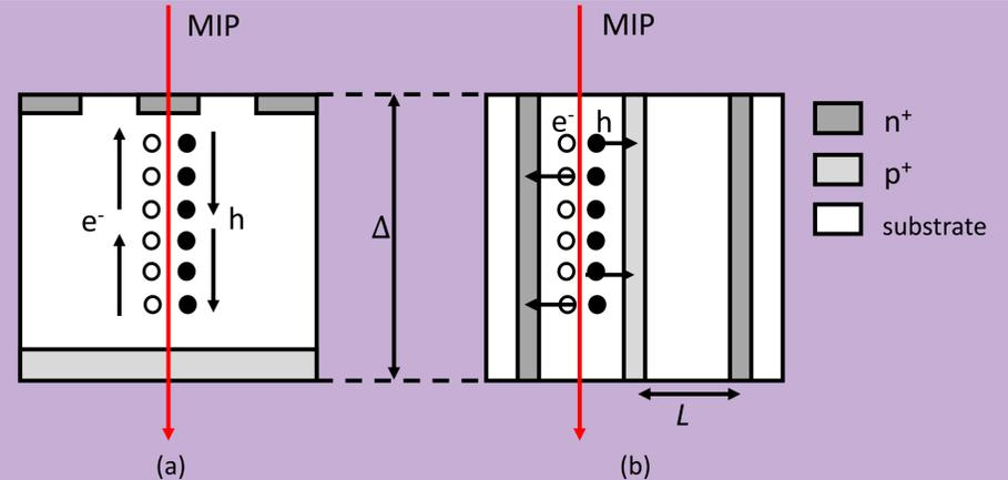
Figure 1: Illustration of the differences in distance travelled by liberated charge carriers in (a) planar sensors, compared with (b) 3D sensors.
