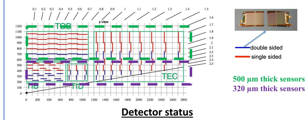
The fraction of active channels of the detector is 96.5%. It remained stable over the LHC Run 2 period. The inactive channels include modules that have no active cooling, 3 control groups that are non-working – one in TIB layer 1, one in TIB layer 2, one in TOB layer 4, few modules that developed HV shorts, following an overpressure incident on the cooling system in 2009.
