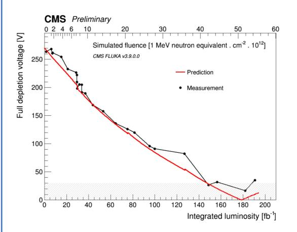
Evolution of the full depletion voltage of a sensor in the first layer of the TIB. The prediction from simulation is superimposed for comparison. It is based on a model which uses fluence and temperature history as inputs [4].
