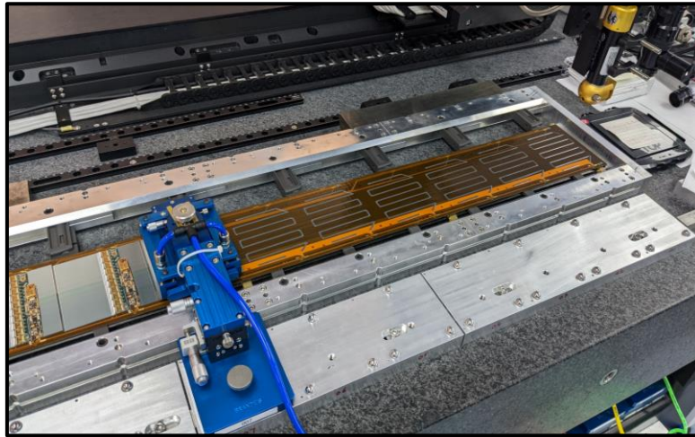
Side J of LS stave being assembled at BNL.
