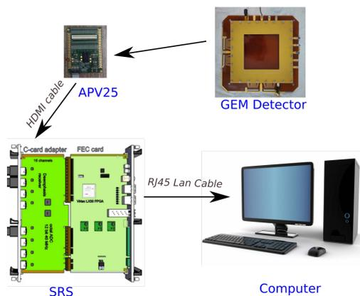
The GEM readout consists of 256 strips running across X and Y-directions, connected to an APV25 Front-end board [4] by 130 pin Panasonic connector. The APV25 has an in-built pre-amplifier and shaper. The charge signals are then sent to Scalable Readout System (SRS) [5] for digitization, zero suppression and further processing. The FEC card present on the SRS handles all the communication, data processing and transfer processes.
