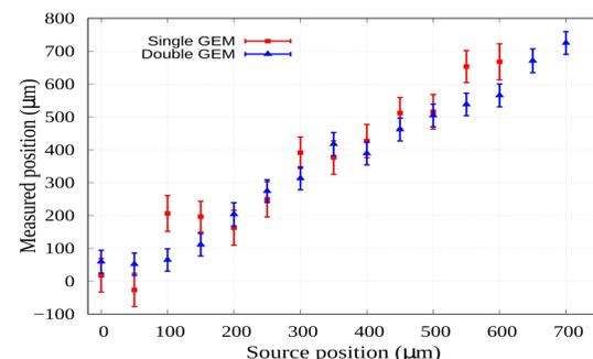
Position information obtained by moving the source in step of 50 μm in x direction.
