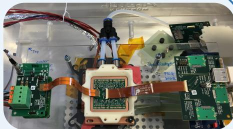
Electrical testing setup for quad ITkPixV1 assemblies
