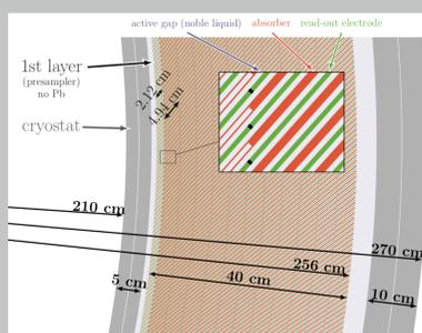
Figure 1: Layout of the proposed FCC-ee noble liquid ECAL barrel in the  $r$ - $\phi$  view.
