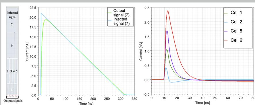
Figure 3: Layout and cell numbering scheme of the readout electrode chunk implemented in FEM tools (left), signal attenuation (middle) and cross-talk current without shield (right).
