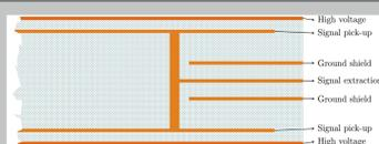
Figure 2: Cross section of the proposed multi-layer PCB readout electrode.
