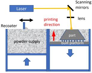
Selective laser melting working principle: recoater spreads a metallic powder bed on built platform, laser selectively melts powder part is build layer by layer (bottom to top)..
