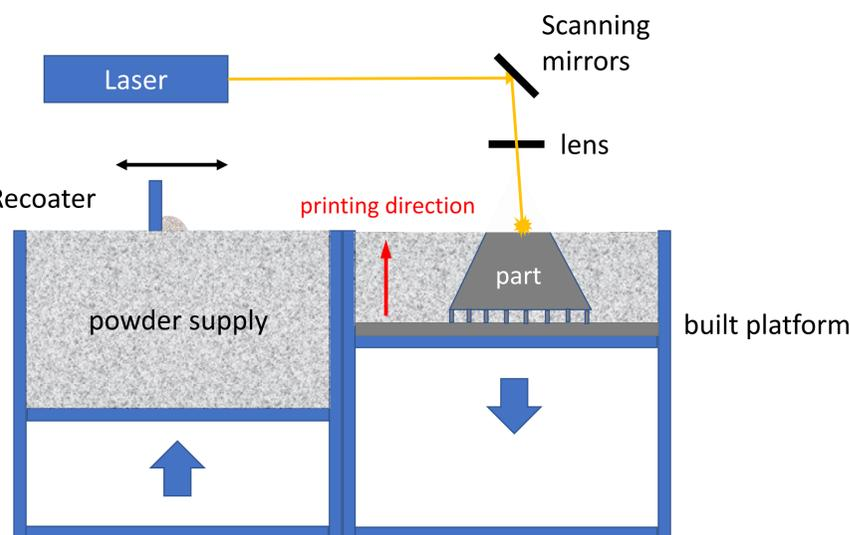
Selective laser melting technology working principle: the recoater spreads a metallic powder bed on the built platform, the laser selectively melts the powder and the part is build layer by layer from bottom to top.
