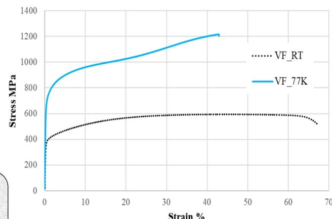
Representative stress-strain diagram of VF sample: RT vs. T = 77K
