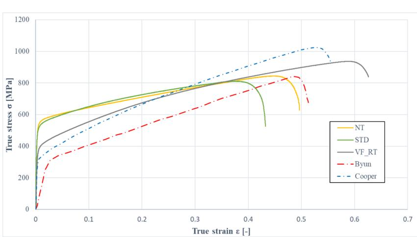
Comparison of true stress strain curves at RT: AISI 316L AM parts subjected to different heat treatment (NT, STD and VF) vs. bulk parts ([1], [2])
