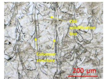
NT & STD → higher  $Rp0.2$  (yield stress) → due to presence of a dendritic structure in the melting pools, consequence of rapid solidification in the AM process.
