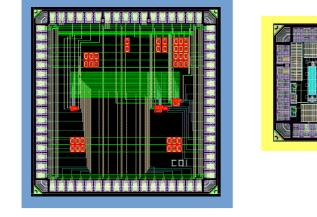
HSI\_ADC01 prototype: evaluation of 4 ADC variants based on SAR architecture: exploring redundancy and switching options.
