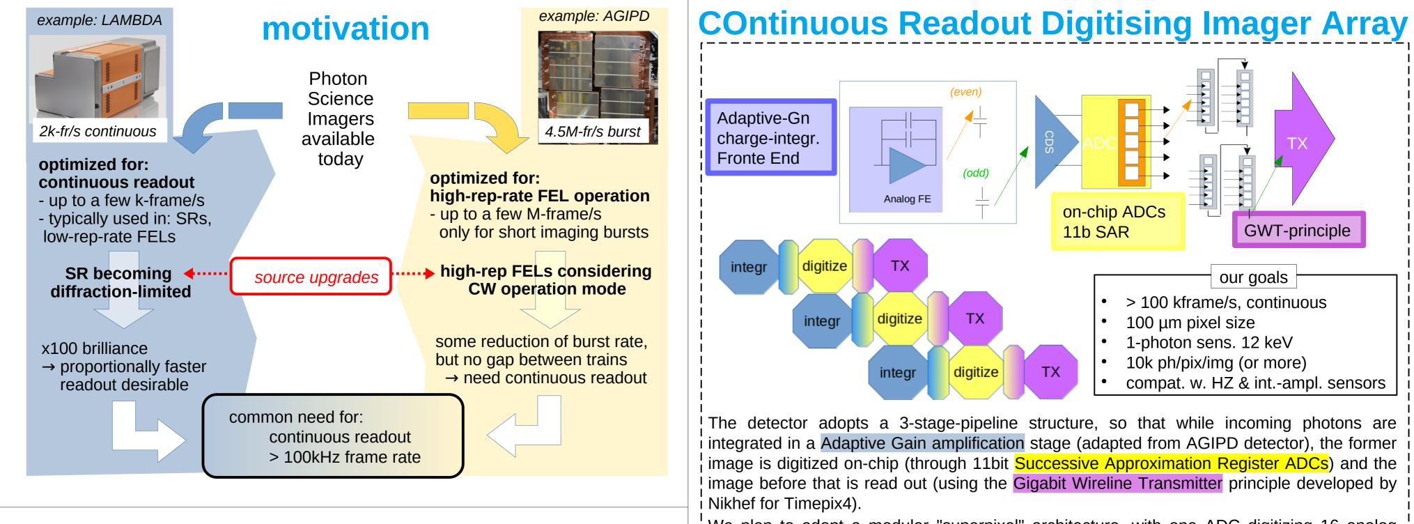
We plan to adopt a modular "superpixel" architecture, with one ADC digitizing 16 analog
