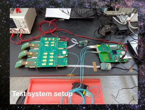
Prior to the PEB prototype, we developed the PEB demonstration system to verify many concerns in advance, such as versatile links, PCB manufacturing techniques, mechanical parameters, key chips, DAQ system, and etc.
