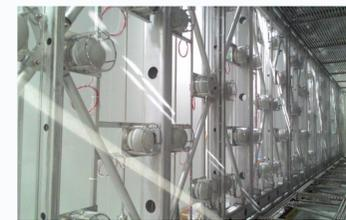
360 HAMAMATSU R5912-MOD (8" diameter) PMTs mounted behind the TPC wire planes.
