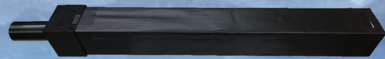
Basic detector element: a 10 cm x 10 cm x 75 cm scintillator bar readout by a 3"-inch PMT
