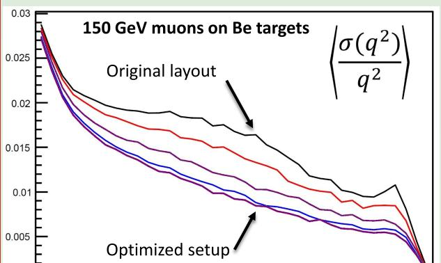
Left: The optimization of the **MUonE** experiment identified a modified layout of its tracker, offering factor of 2 improvement in the relevant figure of merit (relative resolution in q<sup>2</sup> of highenergy scatterings) with respect to original design [1].
