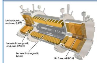
Electromagnetic Barrel (EMB):  $|\eta| < 1.475$ , accordion lead plates
