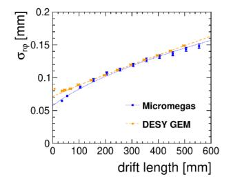
Pad-based readouts show a very similar performance in tracking, dE/dx and double track resolution. ILD-requirements for momentum resolution (∂(1/pt)~10<sup>-4</sup>/GeV/c) can be fulfilled.
