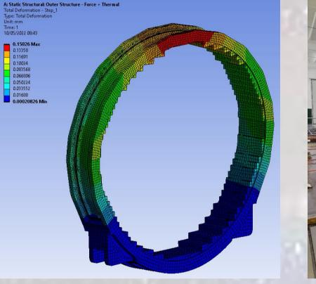
Outer Ring **FEM** Analysis The Outer Ring is a monolithic C-profiled ring and it is machined from a block of aluminum EN AW 6082 T6 to achieve maximum stiffness (max def. 200 microns). FEM analysis shows that the maximum deformation is 150 microns.
