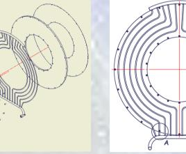
FP under construction **FP** Exploded view FP pipes layout The Back Plate, made of peek, hosts the readout electronics and the SiPM cooling system. SiPMs are thermalized down to -15 °C to minimize dark current and have stable signals.
