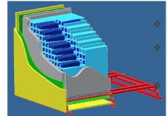
ECal: CsI(TI) crystals + SiPM
