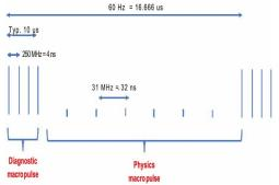
A non-trivial time structure of the beam is required to avoid  $e^+$  beam pile-up in the detector.
