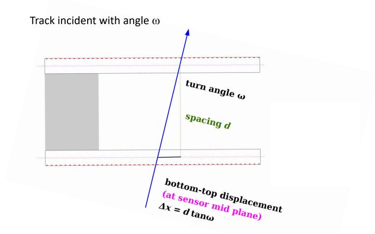
For a spacing = 4.0mm we have a lateral shift of half a strip for angles of 10  $\mu$ m Could gain an effective factor sqrt(2)-2 in resolution *(not yet clear to me the correct gain)*
