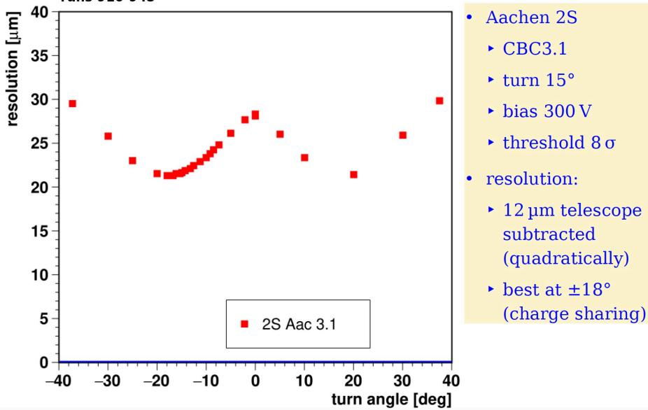
D. Pitzl (DESY): 2S beam test
