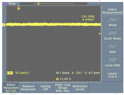
The noise floor at the preamp output with **NO** SiPM connected
