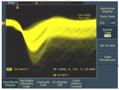
A SiPM signal waveform with SiPM@ -37V
