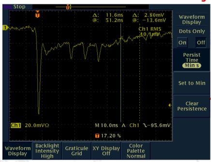
A SiPM signal waveform with SiPM@33V and **NO** "tail cancellation"
