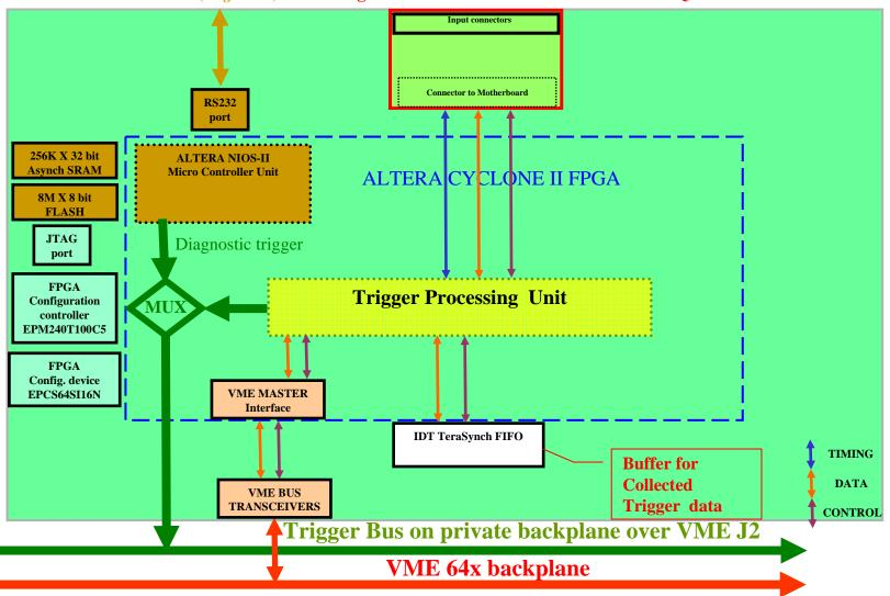
Very Preliminary layout of a BABAR DAQ Interface card for the SUperB IFR Front End: It controls TDC cards and collects data acting like a VME Master with 2e-sst capacity
