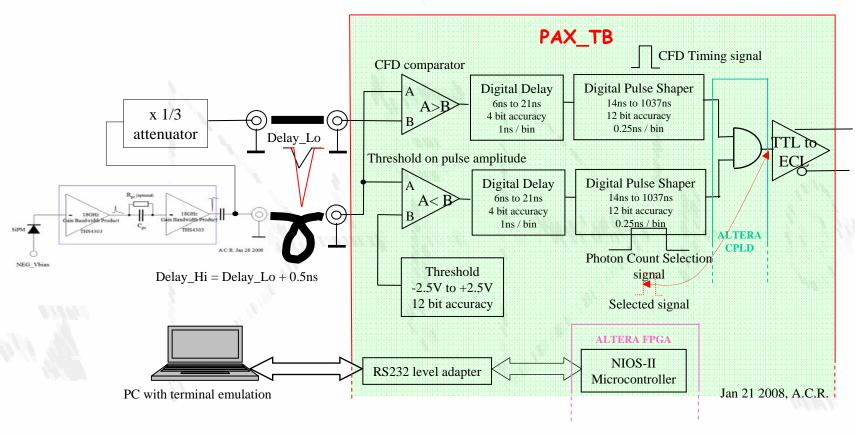
Block diagram of the SiPM signal processing chain proposed here to enhance, if necessary, the time resolution of the discrimination on the SiPM output.
