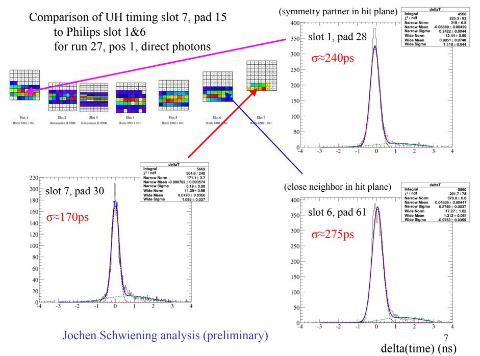
Compare slots as function of position number instead selecting slot 1 pad which is expected to have very similar path length
