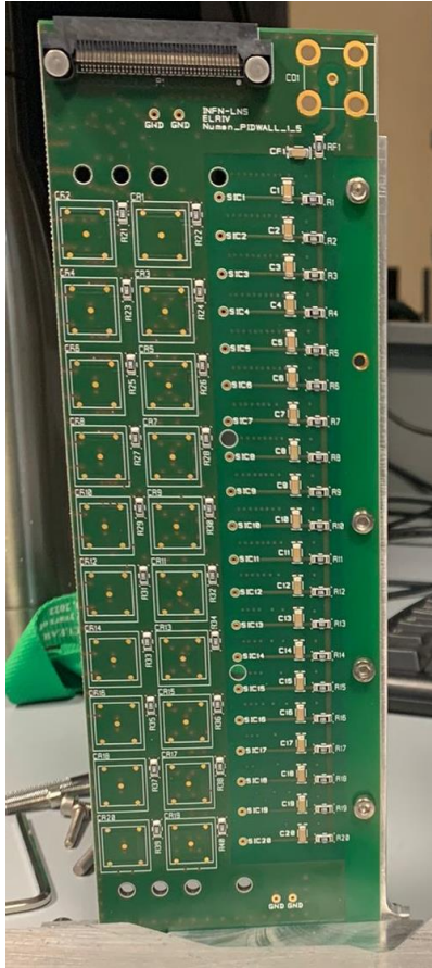
Main PCB for the readout of the detectors
