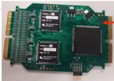
Photograph of the 64 channel SiREAD based (2x SiREAD rev.1) readout card as a building block for the 256 MA-PMT readout.
