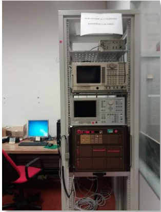
Spectrum analyzer Semiconductor parameter analyzer (HP4156) Switching matrix (Keithley 707)
