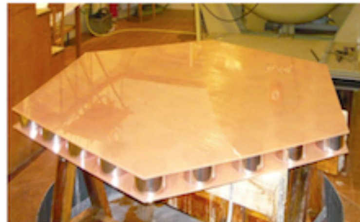
Large Mirror produced in Padua with replica technology
