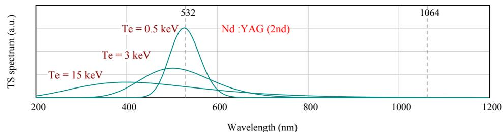
Addition of a second Nd:YAG @ 532 nm extends the measurable  $T_e$  range to 0.1–15 keV
