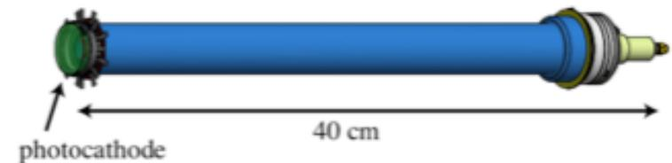
MCP-PMT with S20 photocatode (10mm dia.) and 10 ps resolution (25 x) [10].
