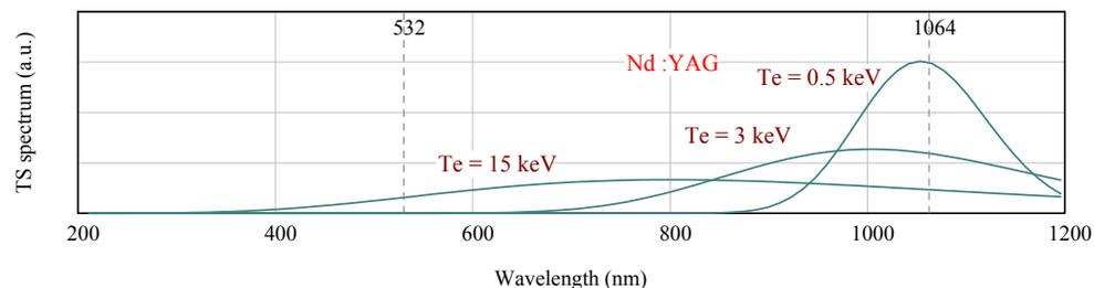
A Nd:YAG laser is the best choice to fulfill the time resolution requirements (2.5 J, 180 ps, 50 Hz) (reliable and commercially available)
