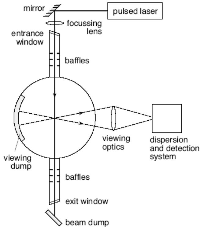
A high power, pulsed laser (3 J, 10 ns, 50 Hz) beam traverses the plasma.
