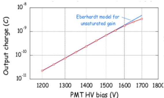
Linearity and gain recovery of JET LIDAR MCP-PMT
