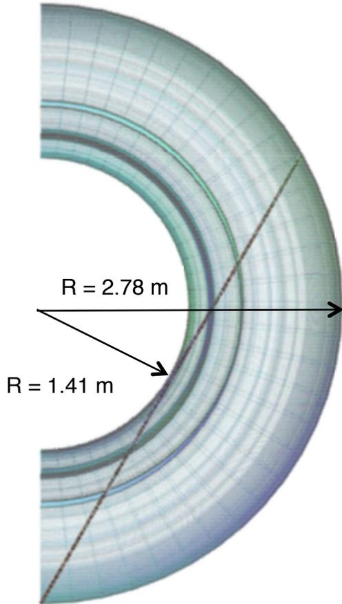
Laser path in the equatorial plane of DTT
