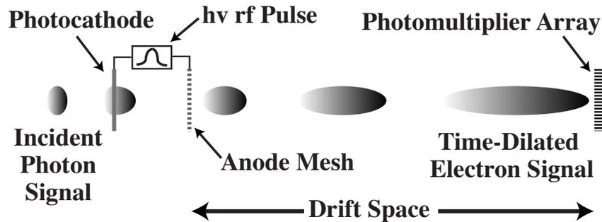
FIG. 1. Principle of pulse-dilation: Photoelectrons are accelerated with a time varying electric field and the resulting energy dispersion causes the signal to stretch axially as it traverses the drift region resulting in reduced effective temporal resolution when sampled with a gated microchannel plate.
