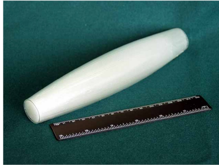
4 th - monolithic lens made of Poly capillaries
