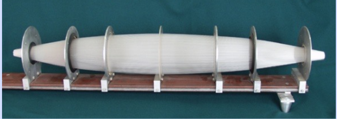
first prototype (handmade) of “Kumakhov lens” \leftrightarrow “Kumakhov optics”
