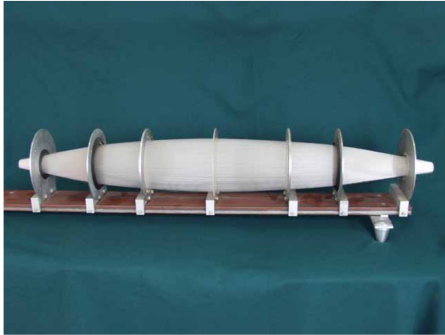
3 rd - assembled lens made of Poly capillaries
