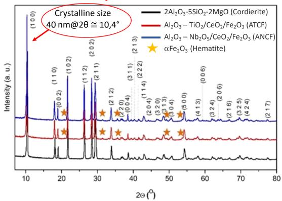
Crystal structure influences the catalyst activity: i.e. in SCRs. the crystalline structure significantly enhances NO<sub>2</sub> formation, causing more rapid selective catalytic reduction (SCR) reactions and greater catalyst reducibility for NOX decomposition
