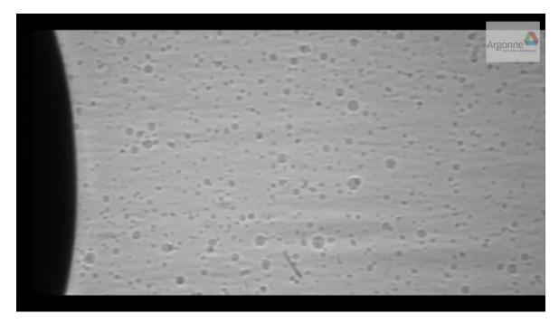
Phase contrast imaging allows time resolved acquisition of sprays inner structure
