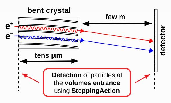
Beam setup in run.mac using GPS commands; all the geometry in DetectorConstruction
