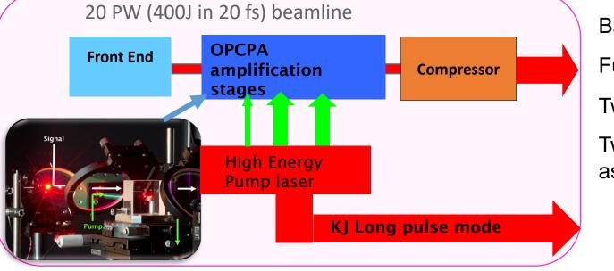
Repetition rate fixed by the pump laser: expected 1 shot / 5 min
