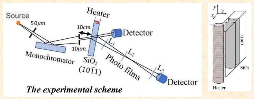
In the experiments, the temperature gradient was applied perpendicular to the reflecting atomic planes ( $10\overline{1}1$ ) of a quartz crystal. To measure the X-rays intensity a scintillation detector was used, and to observe the behavior of focusing at distances of L1, L2, and L3, the frontal section of the X-rays was recorded on photo film.
