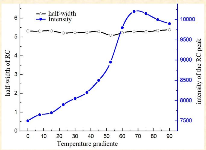
Dependence of the half-width of the RC of  $(10\overline{1}1)$  atomic planes of a quartz crystal and the peak intensity RC on the value of the external temperature gradient.
