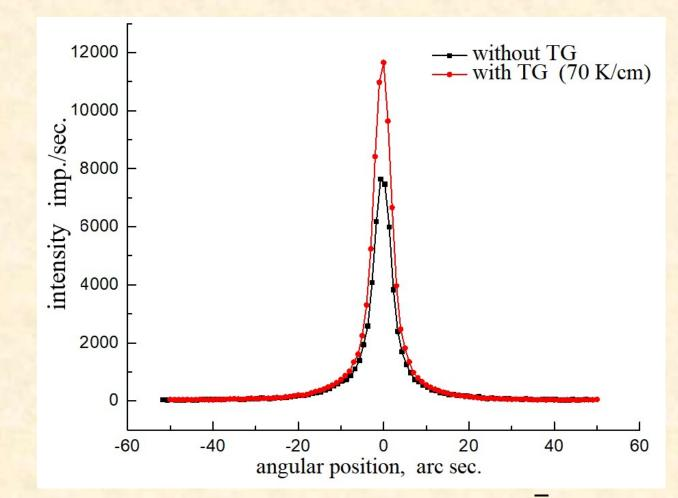
As you see, the half-width of the RC does not change, but the peak intensity RC increases in the presence of a temperature gradient.
