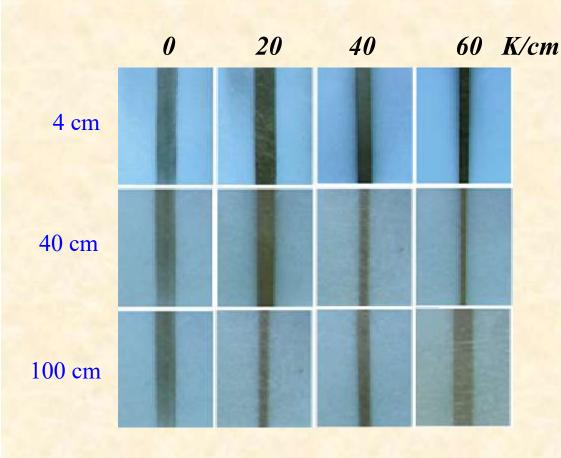
The frontal sections of the reflected X-rays from the reflecting atomic planes (1011) of a single crystal quartz for different values of the temperature gradient.
