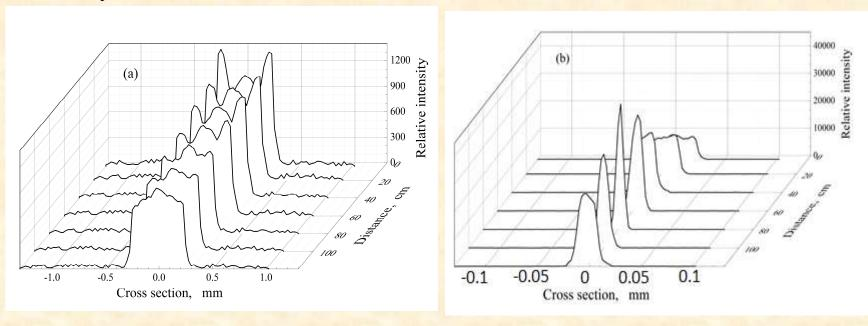
The frontal distribution of the intensity of the reflected X-rays from atomic planes  $(10\overline{1}1)$  of a single quartz crystal of 1 mm thickness at different distances
