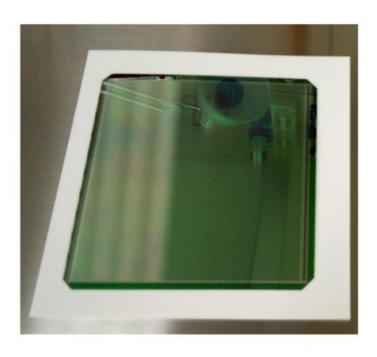
• 150um thick Silicon Sensor from Hamamatsu
