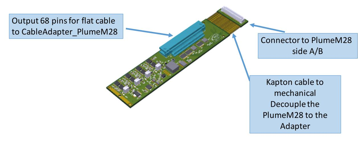
The CableAdapter\_PlumeM28 in production. expected delivery end of January 2020
