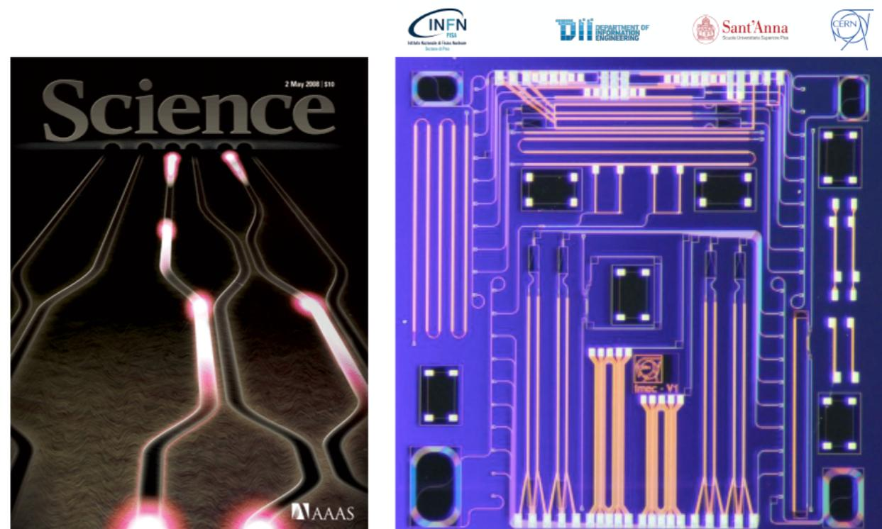
“Graphic representation of an integrated quantum optics controlled-NOT chip. Single photons (represented as flashes) propagate on the chip, confined by silica waveguides, and are then coupled into optical fibers for detection.”
