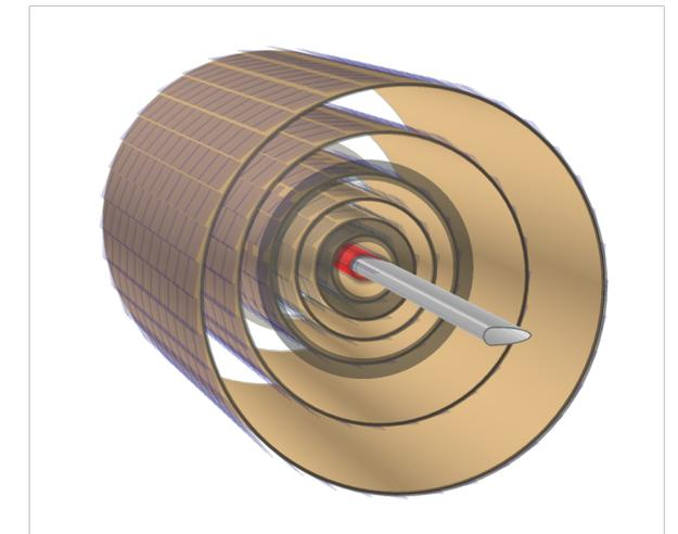
Arrangement of the inner barrel tracker layers around the beam pipe
