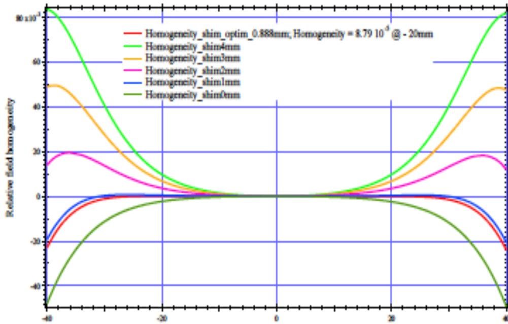
Bending magnets: field homogeneity with optimized shim of  $8.8 \cdot 10^{-5}$  at  $\pm 20$  mm (GFR), better than expected ( $5 \cdot 10^{-4}$ ).
