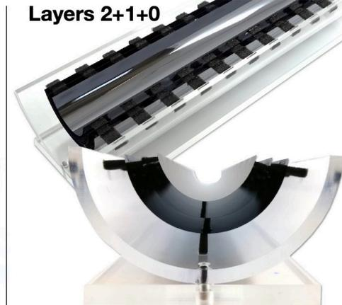
[arxiv:2105.13000](https://arxiv.org/abs/2105.13000) "First demonstration of in-beam performance of bent Monolithic Active Pixel Sensors"
