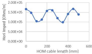
Carefully choose the cable length between HOM window and load help reducing the impedance of 680MHz mode
