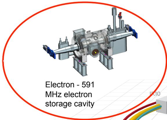
Electron - 591 MHz electron storage cavity
