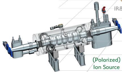
Rapid Cycling Synchrotron - 591 MHz acceleration cavity
