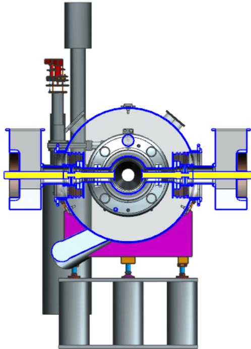
Zoom of one coupler. Pringle position set for minimum  $Q_{\text{ext}}$ . Ceramic in detuned-short position. Courtesy: Jim Henry.
