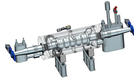
Hadron Cooling - 591 MHz acceleration cavity
