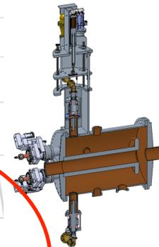
Hadron - 49.2 MHz and 98.5 MHz bunch splitter cavity
