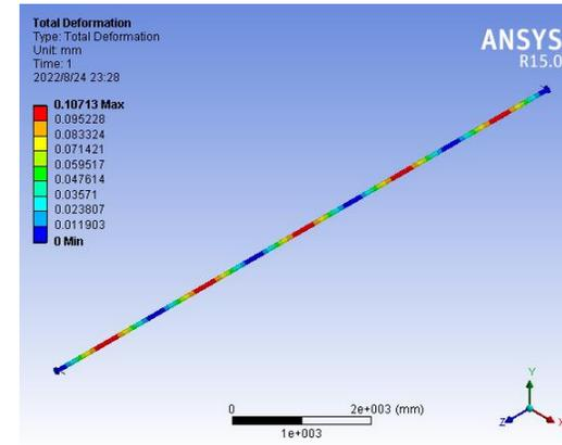
Every 2m is supported, with a maximum deformation of 0.1mm
