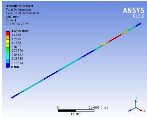
Every 3m is supported, with a maximum deformation of 1.66mm;
