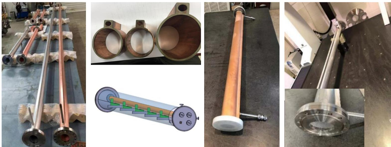
Round chamber is easier to be fabricated.
