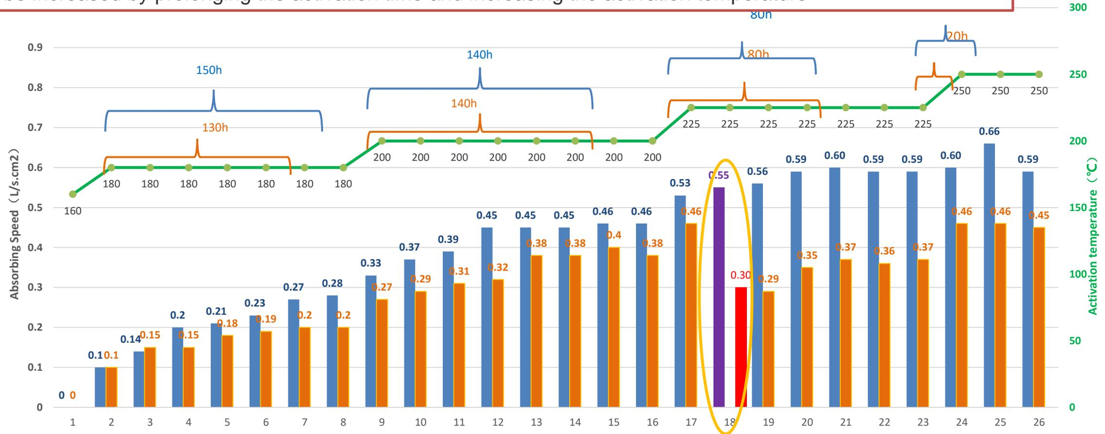
No63 is the number of NEG coating, (2),(3) represent the two different NEG coating pipes at the same coating process
