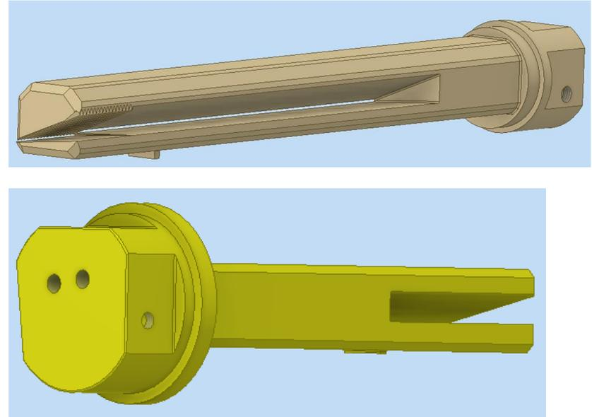
Photon absorbers bear ~85% of the synchrotron radiation power:
