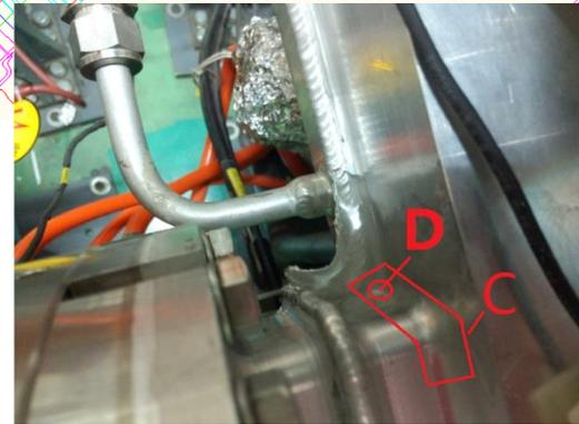
**Review:** The leak location was similar to the first leak for material defect on Aug.20 2013.
