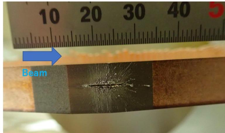
Damaged tip of D09V1 (KEKB type) in HER due to the sudden beam loss
