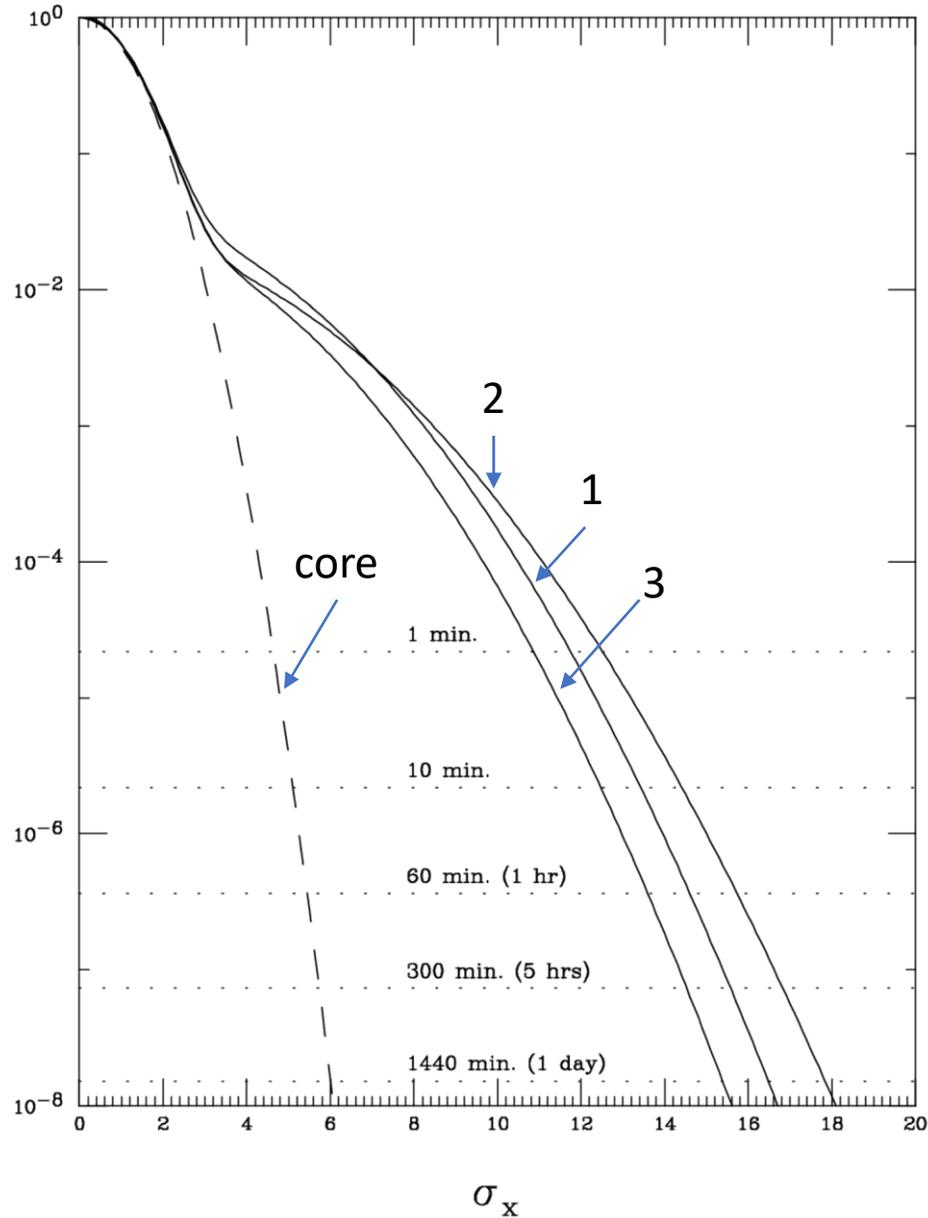
Tail distributions that can generate the background level seen in the superKEKB pixel detector (PXD) during early running.
