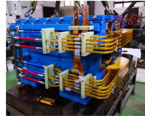
The mechanical design of a full size CEPC collider ring dual aperture dipole of 5.7m long has been designed and be fabricated at the end of 2021.
