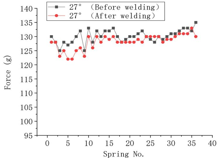
Contact force is identical in different fingers and meets the requirement of  $125 \pm 25g$ .
