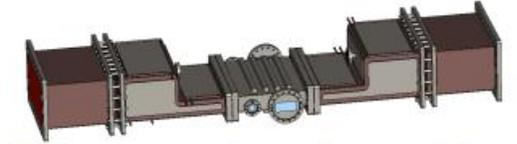
High power test scheme of output window
