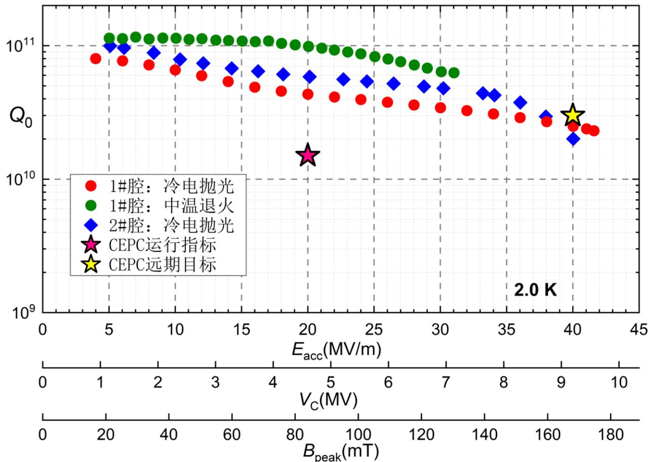
650 MHz single-cell SRF cavity test results
