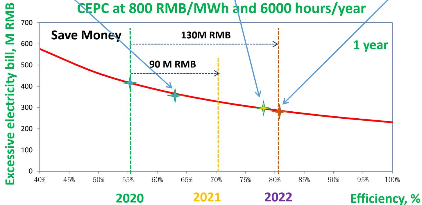
Efficiency impact on operation cost (Only considering operation efficiency of 650MHz klystrons)
