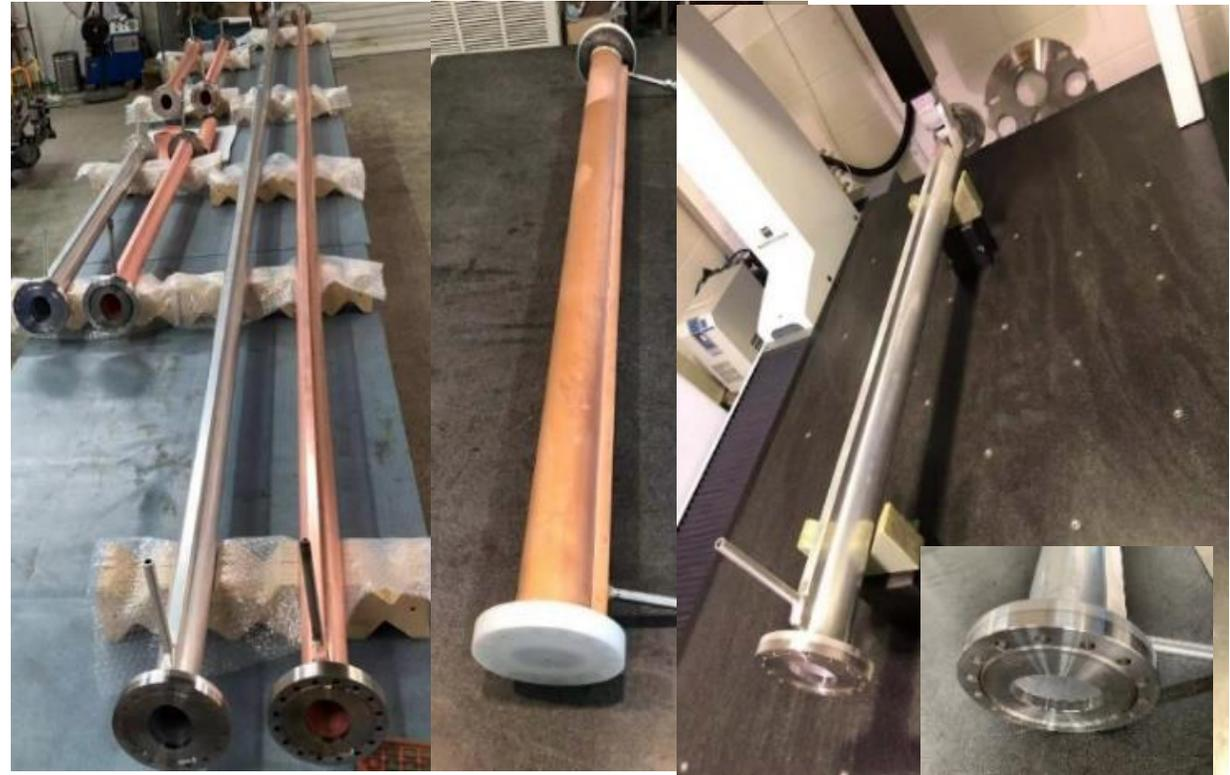
Elliptical and round vacuum chambers have been made
